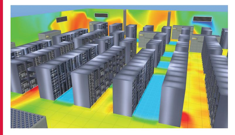
A TileFlow<sup>®</sup> model gives you detailed information about the airflow, temperatures, and pressures throughout the data center. You can use this knowledge to:
